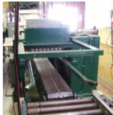
A POWERED DRUM DIBBLER.
