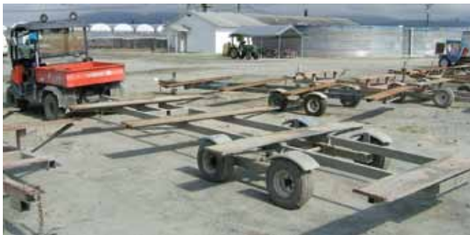
CUSTOM BUILT TRAILERS FOR MOVING COPPERBLOCKS TRAYS ON CUSTOM PALLET
