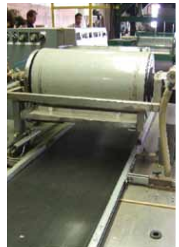
VACUUM DRUM SEEDER – SINGLE REVOLUTION PER COPPERBLOCK
