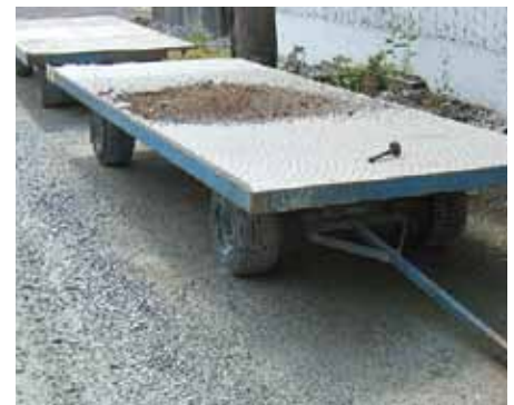
PNEUMATIC TIRED TRAILERS, HOLD 100 COPPERBLOCK TRAYS EACH.
