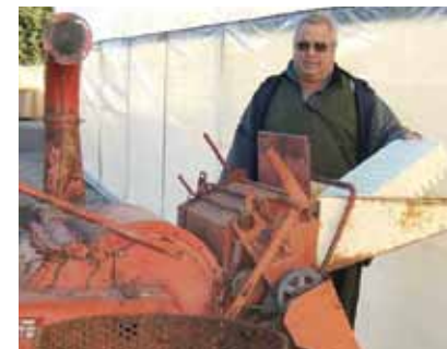
BILL BOERBOOM OF MOUNTAIN VIEW GROWERS INC., SUMMERLAND BC, USES AN OLD CORN GRINDER TO PRODUCE STYROLITE MEDIA AMENDMENT ON SITE.
