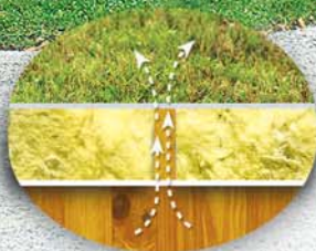
Heat Transmitted through Framing Members
